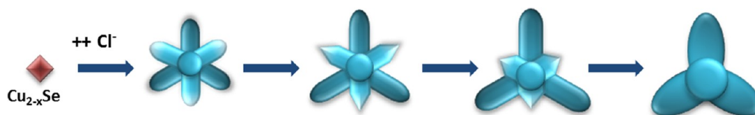
Scheme 1. Typical evolution of the CdSe/CdS multipod shape when large molar fractions of CdCl 2 are introduced in the synthesis of core–shell CdSe/CdS NCs, starting from Cu 2–x Se as seeds. After the cation exchange reaction, during which the Cu 2–x Se NCs are converted into CdSe NCs, octapods are first generated. Soon, however, in many of these octapods, the four pods with sharp tips start receding and eventually disappear. The other group of pods instead keeps growing, such that many NCs are reshaped into tetrapods.
